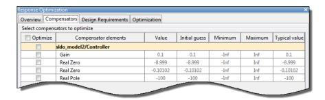
The **Compensators** tab displays the following parameter settings:
