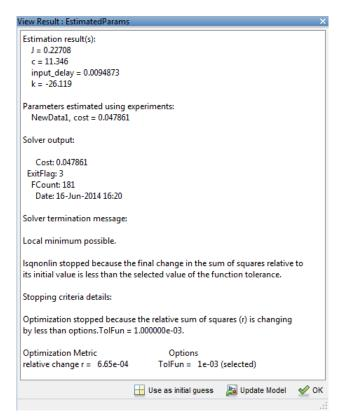
Examine the estimated cost function graph. Cost function is the error between the simulated and measured output. During estimation, the default optimization method Nonlinear least squares, lsqnonlin, minimizes the cost function by changing the parameter values. The following figure displays the change in the expected cost during iterations.
