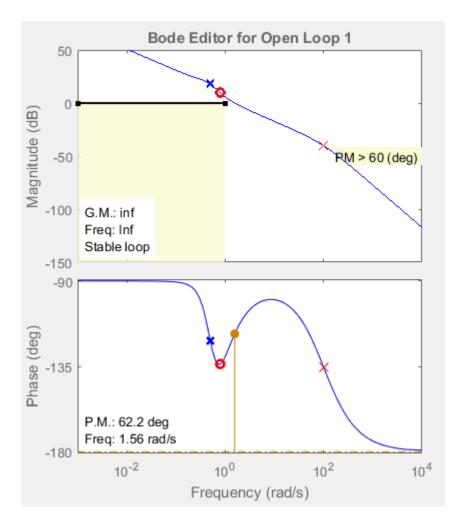
Verify that the closed-loop response of the system remains stable after refining the controller design.
