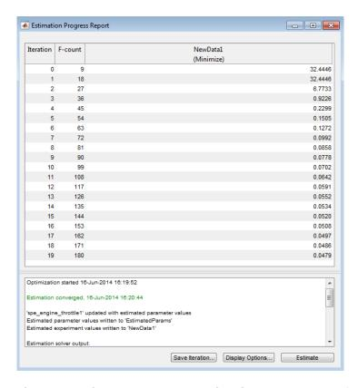
The estimated parameters are saved in the **Parameter Estimator**, in the **Results** section of the **Data Browser** pane, as EstimatedParams. Right-click EstimatedParams, and select **Open...** to view the results.
